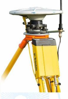
1 no. Trimble R750 CORS Antenna (Modular GNSS Receiver)
